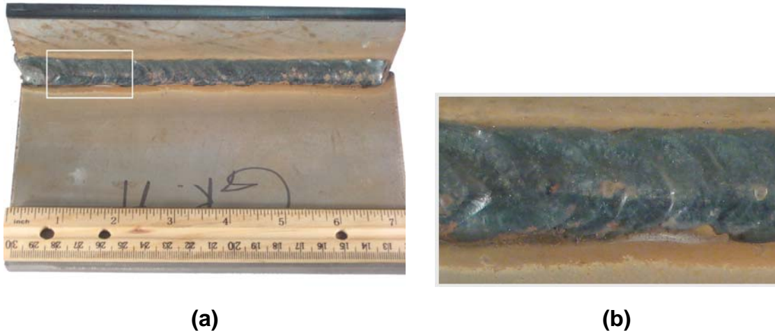
Figure 20 Initial condition of ABS-A plates joined at 90 degrees (a) overall view of weld bead and (b) inset view of weld pool segment.
